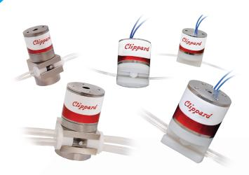
NPV series pinch valves are solenoid-operated devices that are designed to open and close tubes for controlling flow of liquids and gases. Whereas other valve types have internal passages that may cause small amounts of fluid to remain in the valve, pinch valves have no areas where fluid can become trapped. Energizing the solenoid retracts or attracts the plunger, which opens or closes the tube, while de-energizing the solenoid allows the plunger to return to its original state.
