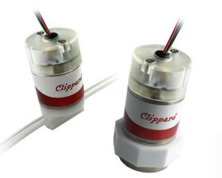
The general principal behind a hit and hold circuit is that the valve is energized to full power for a short period of time before dropping the voltage and current to a specified level. Applications that are sensitive to heat rise can greatly benefit from hit and hold circuits, as can high cycle and low temperature applications. In some applications, hit and hold can actually extend the life of the valve.
