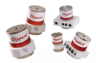
The NIV series media isolation valve is a solenoid-operated device that utilizes a flexible diaphragm to isolate the actuation mechanism from the fluid path. This unique, addition, all wetted areas of the NIV series are PTFE, making
