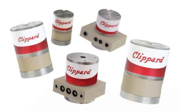
The PIV series features the same solenoid-operation and multifunctional valve stem design as the NIV series but with the added benefit of a PEEK body. This enables the PIV series to deliver higher pressures and provide enhanced durability. All wetted areas of the PIV series are PTFE and PEEK.
